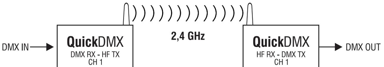
The DMX signal is fed to a transmitter which sends it via RF. A receiver with the same transmission channel receives the RF signal and distributes it as a DMX signal.
